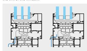
Concealed drainage versus traditional drainage through the frame profile and drainage caps  $% \left( 1\right) =\left( 1\right) \left( 1$
